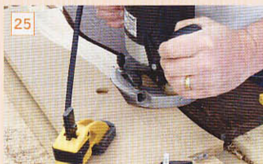
25 Working from right to left, keep the router tight up against the fence
