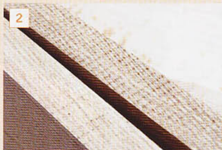
2 Small ripples left by the blade are sometimes enough to accentuate the glue line
