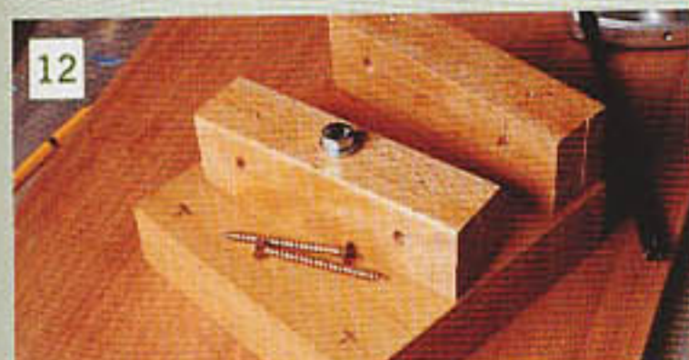
12 The bolt needs to be sawn to length so it secures the top and bottom halves of the front support block without being able to screw in far enough to foul the saw table while in use
