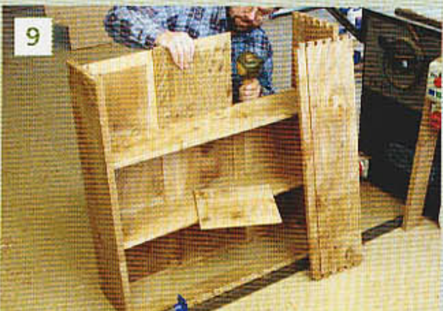
9 The cabinet is dry-fitted as a trial run
