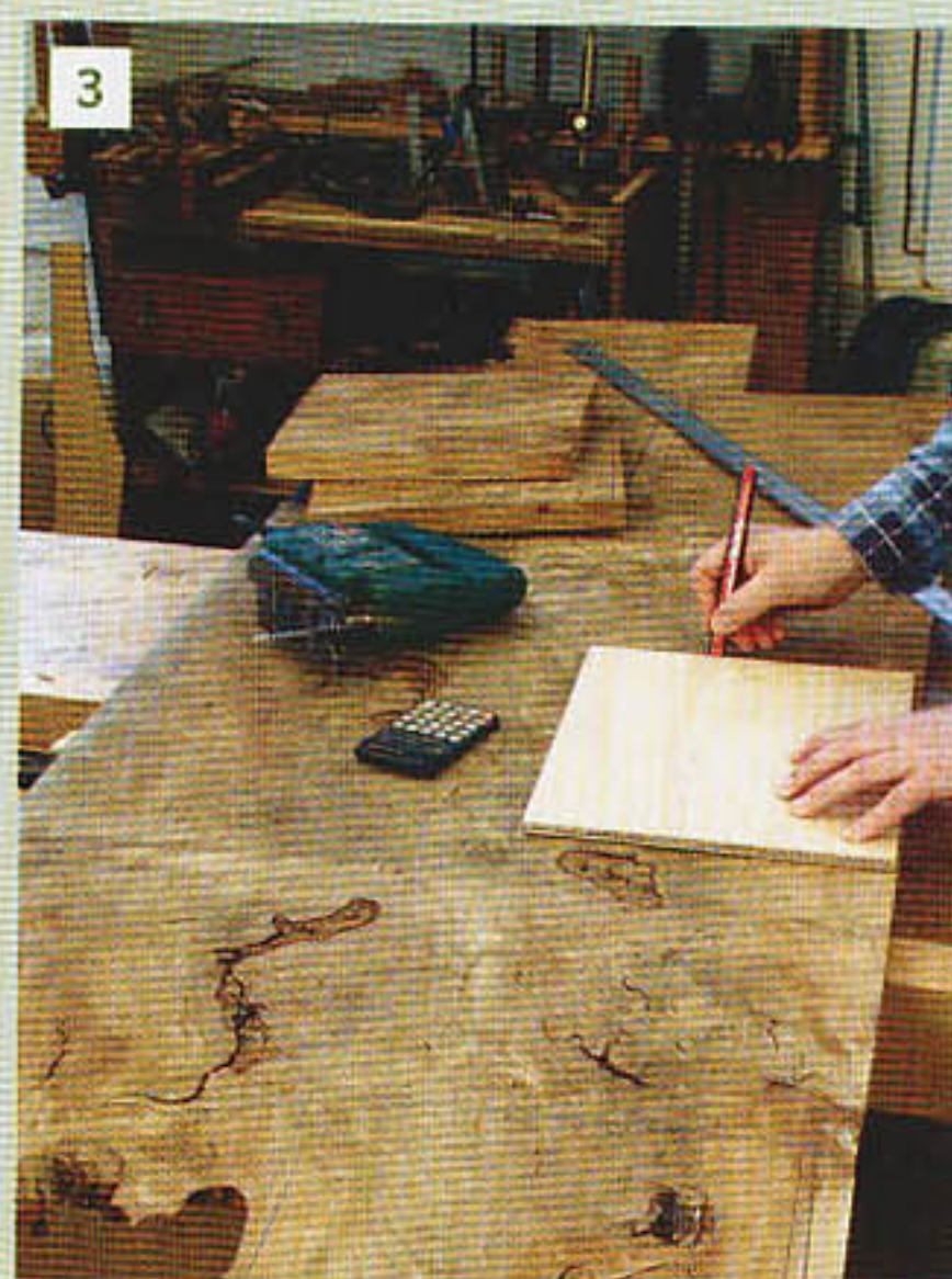
3 The panels are marked out with a template and cut from between major 'natural features' in the elm
