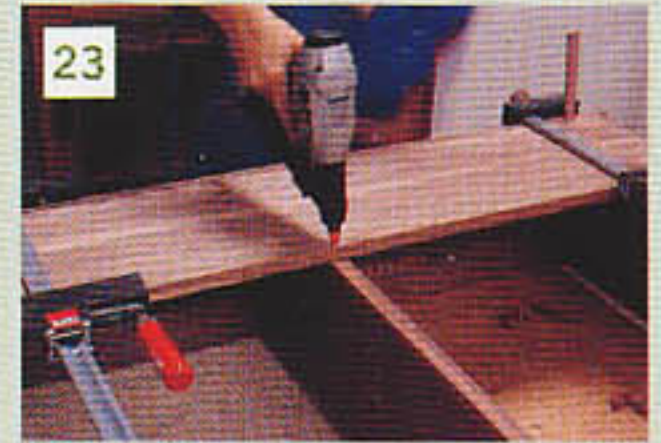
23 Nailing the backboards in position
