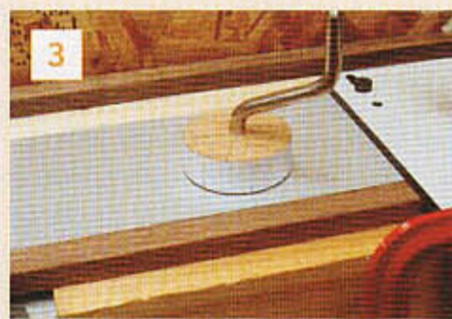
3 A paper scale divides up the wheel into seven equal segments
