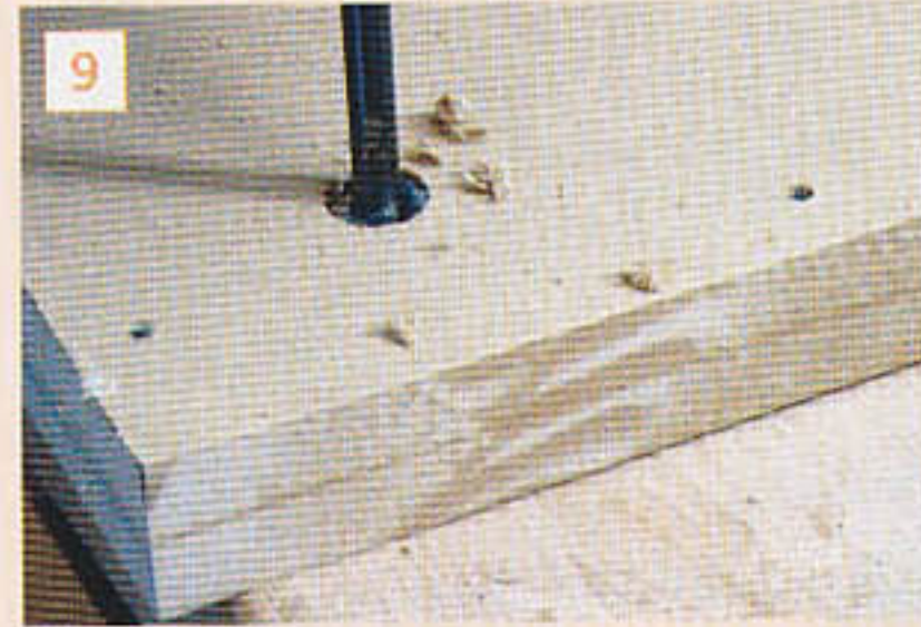
Counterbore the underneath of the jig so the heads of the coach bolts are flush with the base
