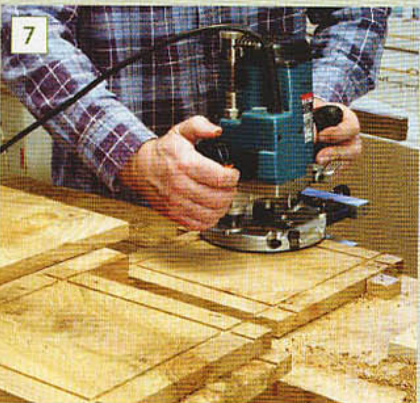
7 Fielding edges are pre-routed with a straight bit
