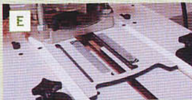
A single pull through makes the cut. There is no need to cut a clearance housing first
