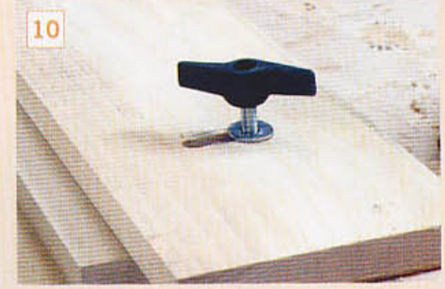
The clamping arrangement is some form of locking handle or knob
