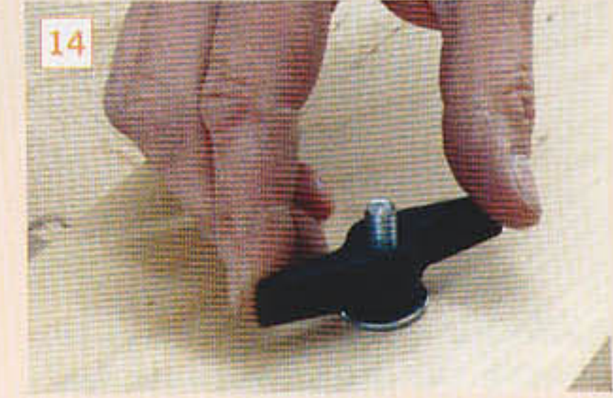
Clamp one of the pieces you wish to trim under the fence
