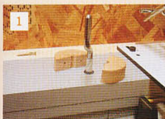
1 The indexing wheel is fitted to the crank handle. The tape ensures a tight fit with no risk of slipping
