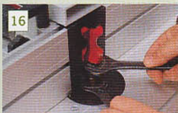
16 Installing the cutter for the partial bull nose of the top. The collet extension makes this easier, but only if it is well balanced and the cutter is not removing large amounts of material
