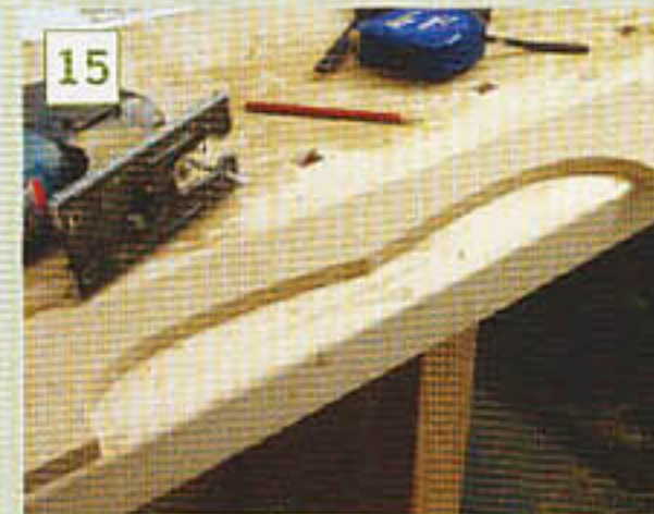
15 Use a jigsaw with a fine blade to minimise any tearing
