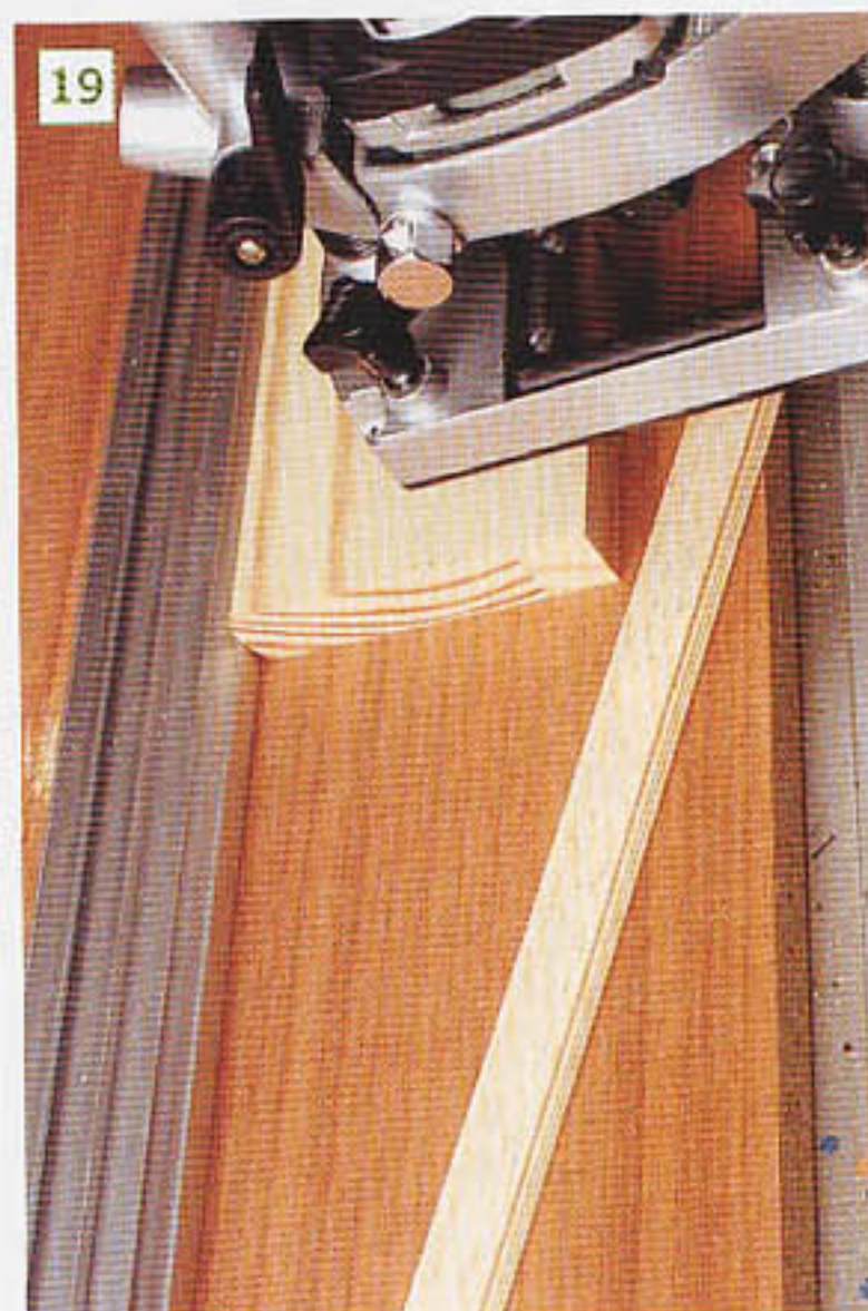
17 Setting up the router with a 1/2th scale skirting board cutter from the Trend dolls' house cutter set
