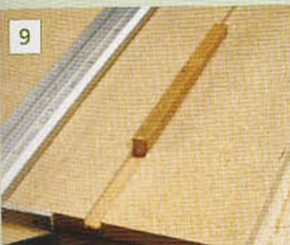
9 Use a small offcut of the shelf material to lock the sides together
