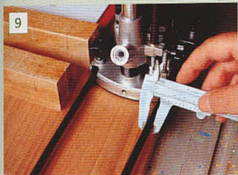
9 Check the diameter of the guide rods of the router to ensure the correct-size drill bit is selected for a fairly tight fit
