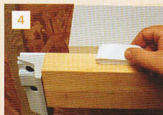
4 Double-sided tape will hold the stock in position
