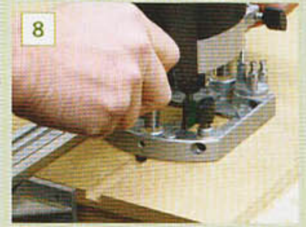
8 Make sure you run the router the right way
