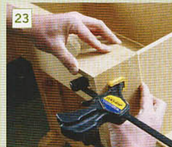
23 Once the carcass is dry fix the plinth in place
