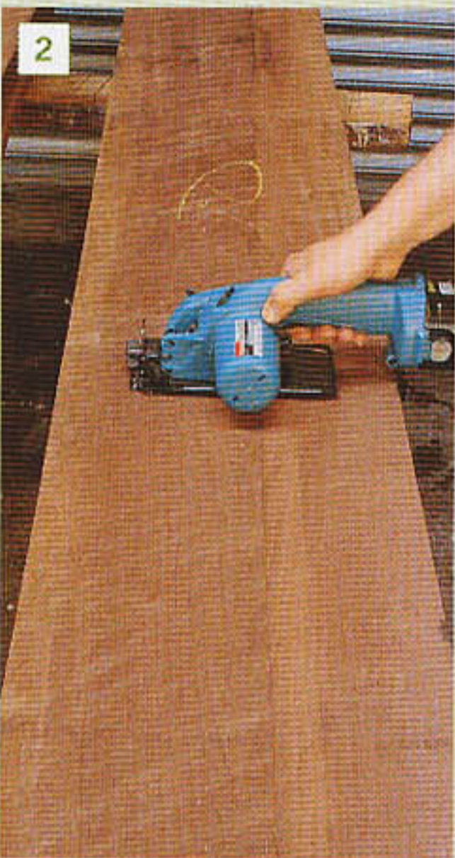
2 This little Makita cordless saw has a big heart and is more than capable of cutting this inch thick walnut down to size
