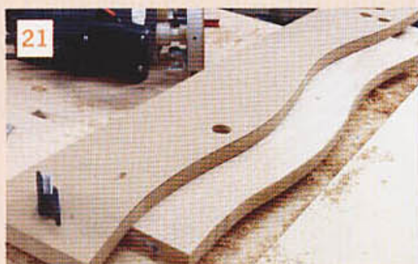
21 Make sure the line of the curve is all within the gap between the two pieces of the table
