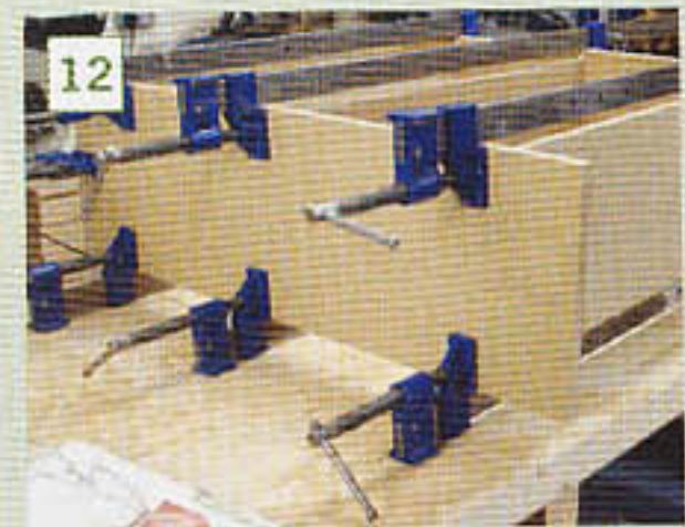
12 Glue up the carcass using more glue than normal
