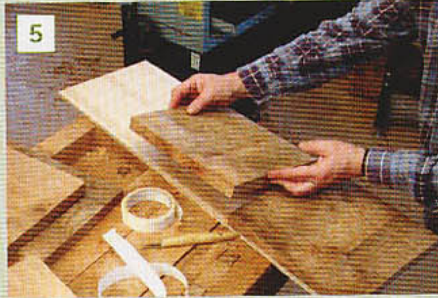
5 The panels are taped on a 'sledge' board ready for thickening
