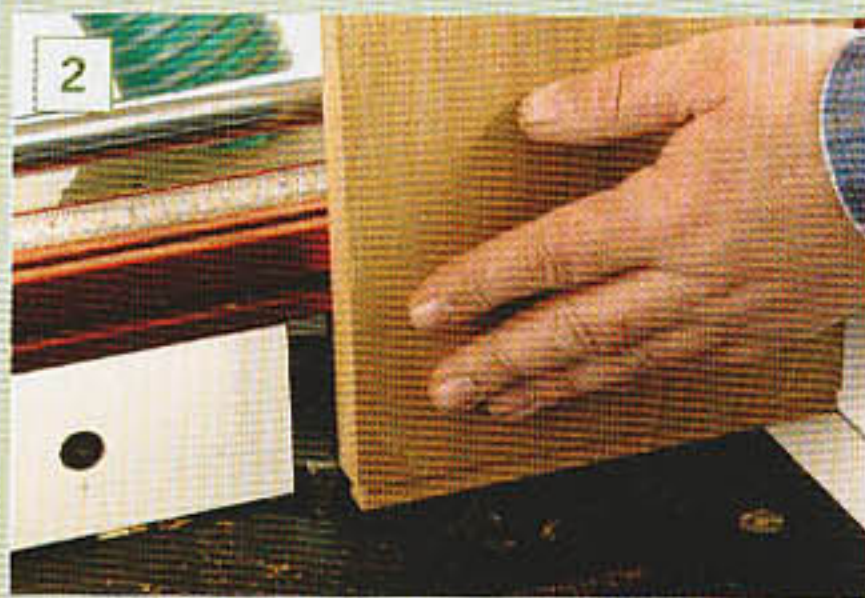
2 The dovetails are routed on the shelf ends to slide into dovetail housings
