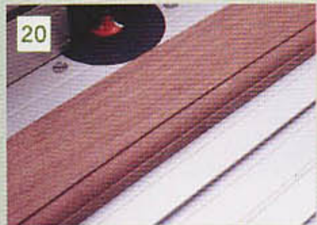
20 ...and run some moulding for the plinth
