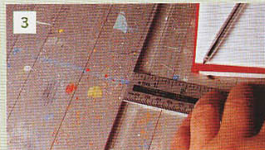
3 Check the dimensions of the saw table guide slot before cutting the guide strip for the sliding baseboard
