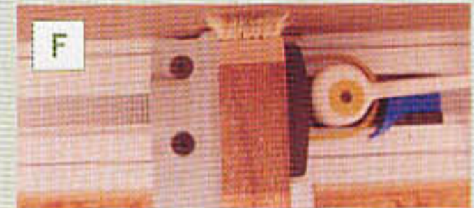
The nail brush on a stick is used to apply pressure to the underside of the board and keep the top surface in contact with the underside of the baseplate
