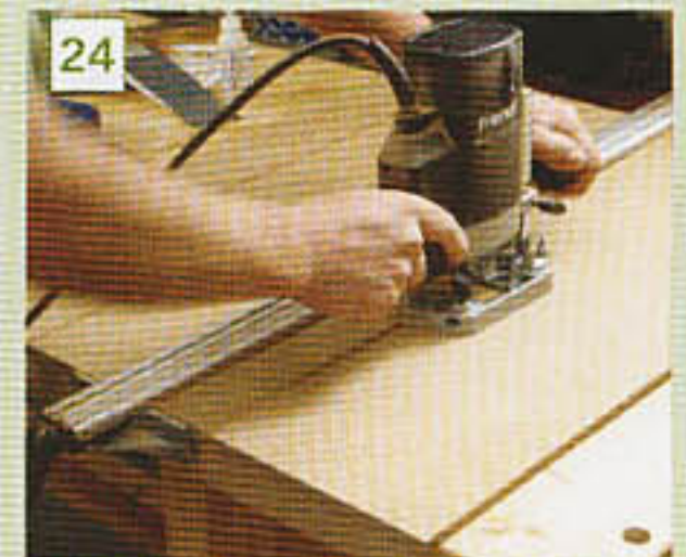
24 A series of V-grooves cut to imitate match boarding
