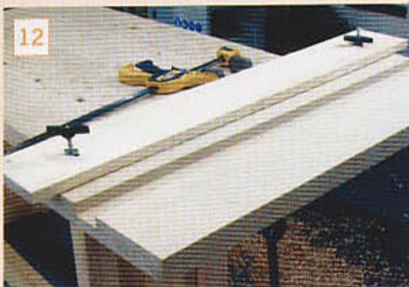
That is all there is to this simple edging jig
