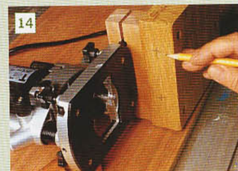
14 Mark the hole positions for the screws which will attach the support block to the saw table rip fence
