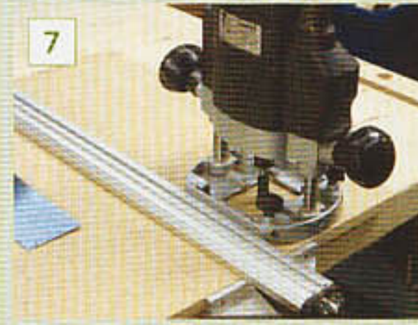
7 Clamp the straightedge across both boards and rout them as one
