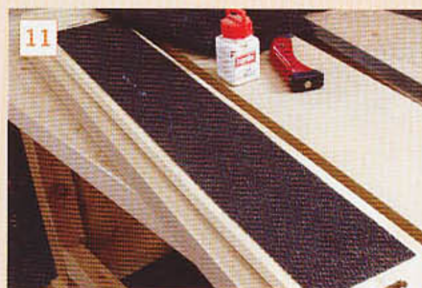
11 I stuck a strip of non-slip mat to the underside of the fence
