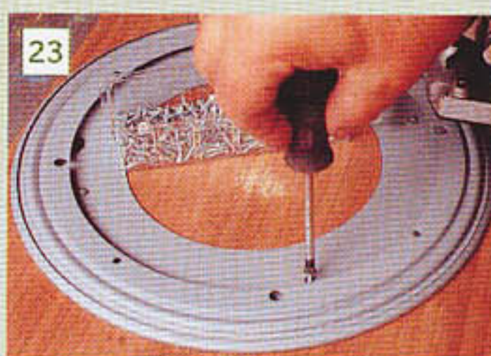
23 The bearing is screwed down onto the main baseboard
