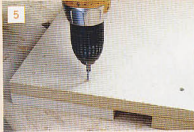
Glue and screw the two parts of the table onto the baseboard
