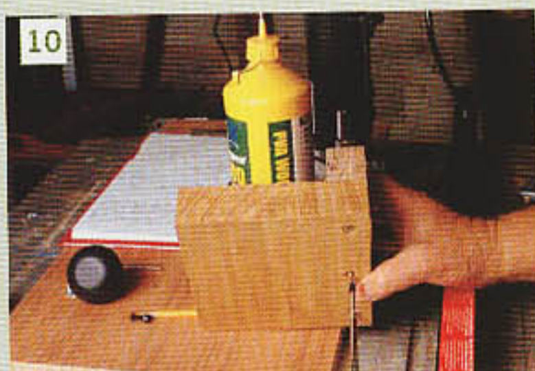
10 Fitting the rear rod support block with glue and screws
