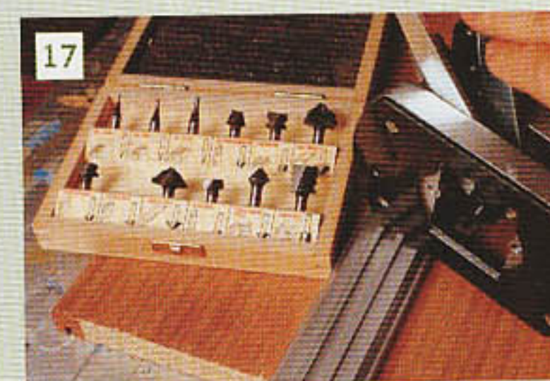
17 Setting up the router with a 1/2th scale skirting board cutter from the Trend dolls' house cutter set
