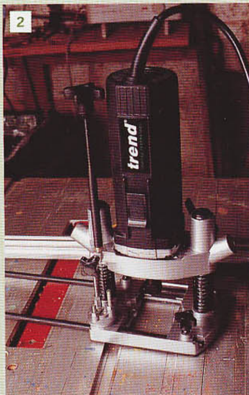
2 Guide rods and a fine height-adjuster fitted to the T3 router ready for installation
