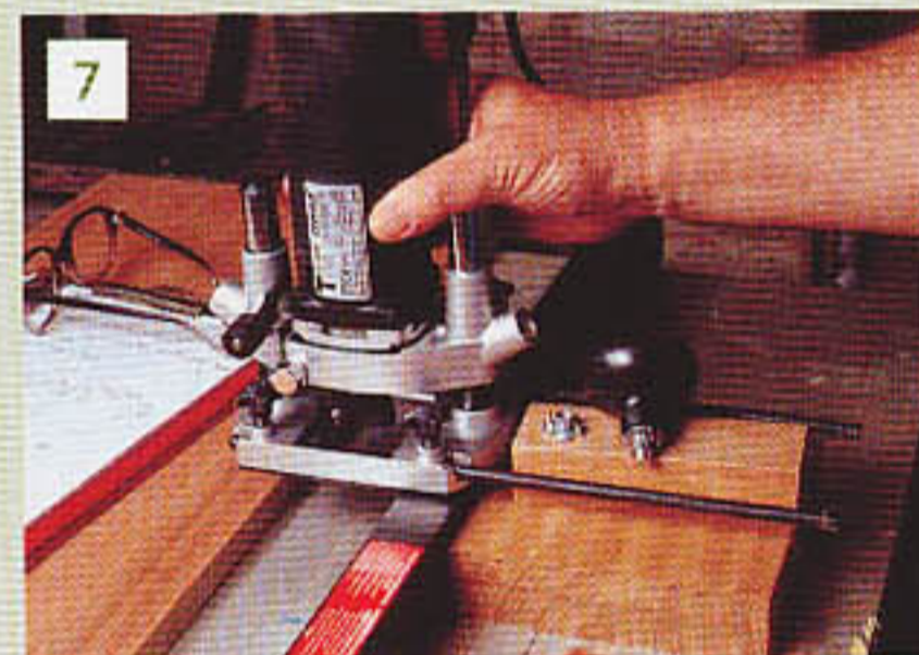
7 Check that the router to be installed fits into its main support block. Note that the router base partially rests on the rip fence for additional support and stability
