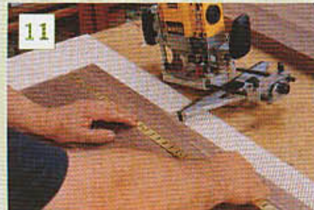
11 The recesses are cut the full length of the sides and a final check for fit is made
