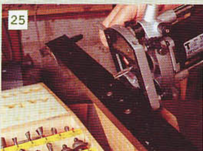
25 Fitting a straight cutting bit to the router which will be set up in its support block and used to cut the rotating baseboard in a circle which will exactly match the operating position of the router
