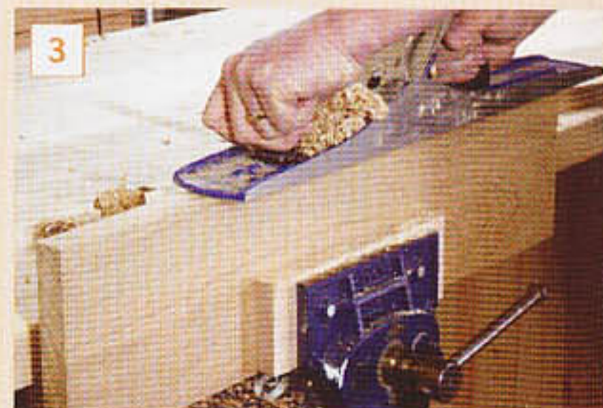
3 Traditionally the use of a long-sole plane was the only sure way of truing up the edge
