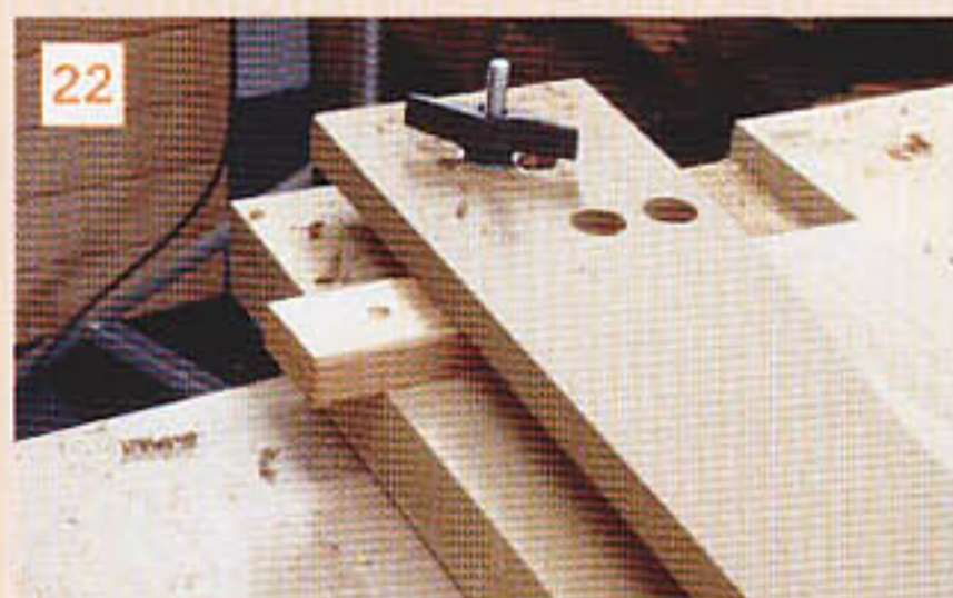
22 Use a temporary packing piece to stop the fence tipping backwards
