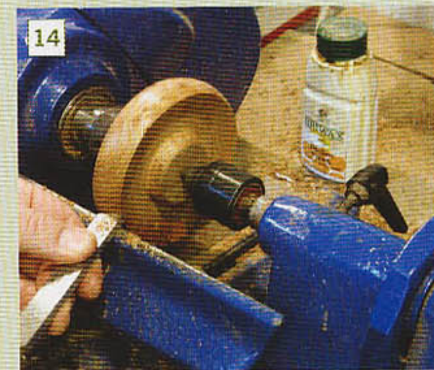
14 Door pull handles turned as a disk, then sliced off
