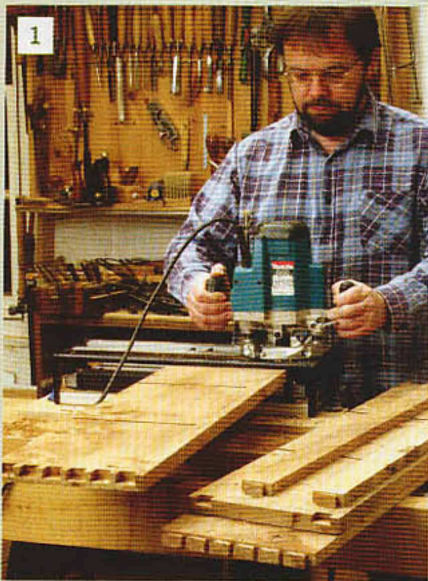
1 The carcass is dovetail-jointed on the corners
