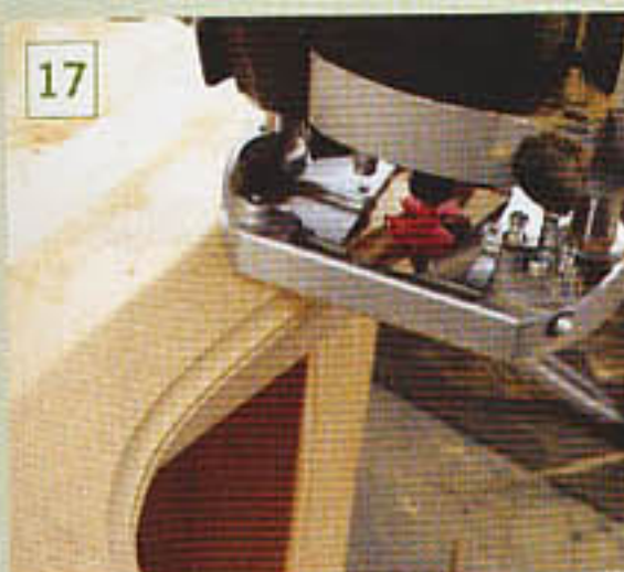
17 Run a bearing-guided cutter around the shape
