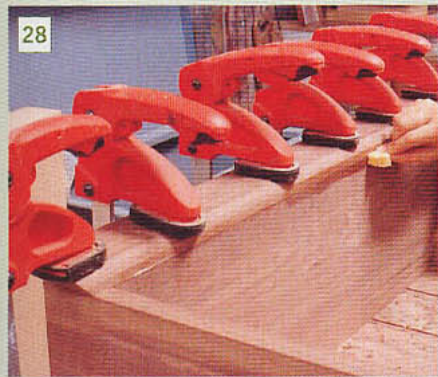
28 Cramping the front of the plinth to the bottom shelf
