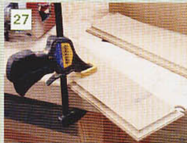
27 The same technique is used for the drawer fronts which are planted onto the front of the drawer
