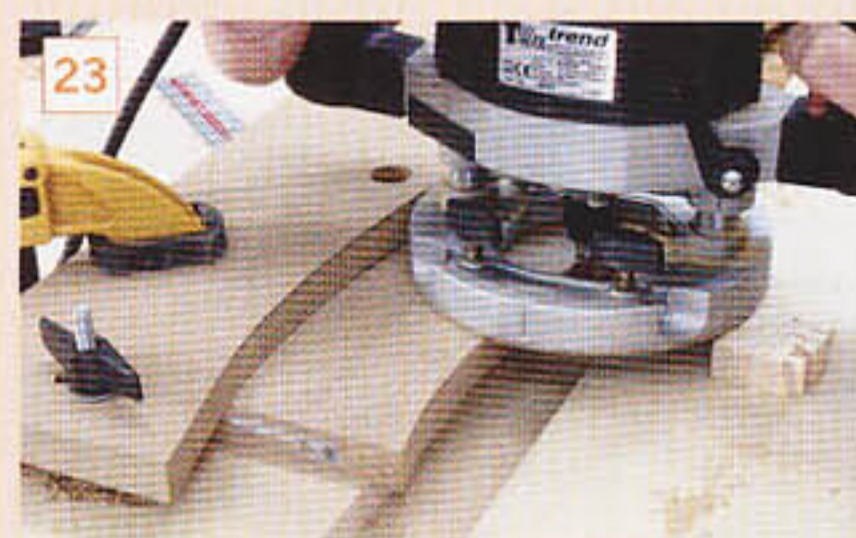
23 Now use the round part of the base to run against the fence
