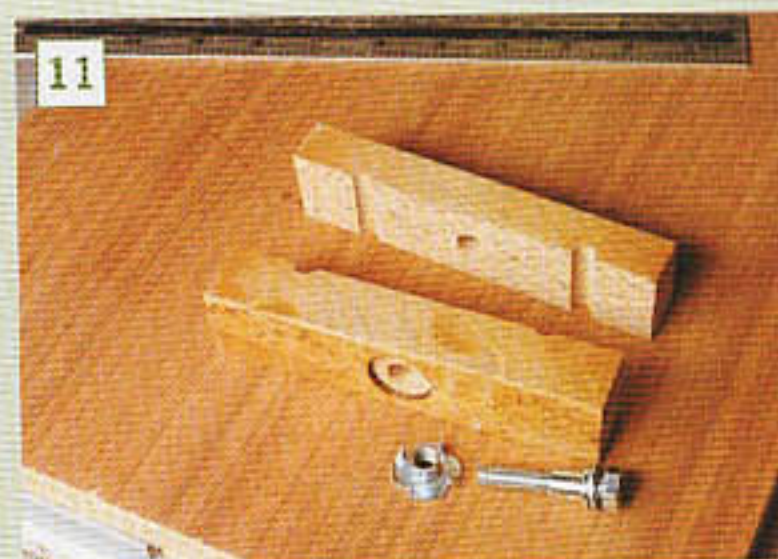
11 Saw the front support block in two halves and have the prong nut ready for installation
