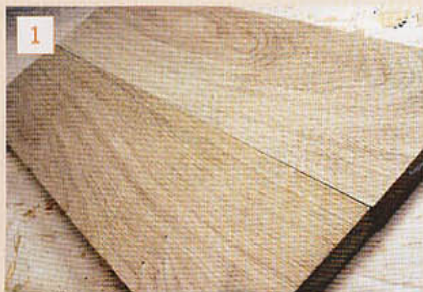
1 There always seems to be a gap at either end of the joint
