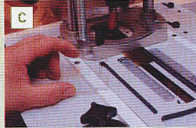
Once the depth of the dovetail is set, make a template of the shape of the housing in a piece of clear acrylic. This will be used later to fit the dovetail to the housing
